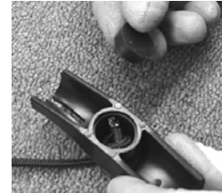
Remove the plug in the handle. Untie the knot in the rope. Slip the rope out of the handle.
